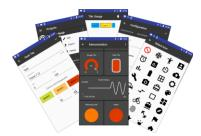
A free iOS and Android app is available to download, which enables users to create dashboards with varying degree of detail based on application requirement. It enables B24 systems to be visualised on phones and tablets by using digital displays, gauges, tanks and charts. Displayed data can be defined as mathematical expressions consisting of readings from multiple transmitters, functions and constants. The app also facilitates B24 module configuration and calibration.
