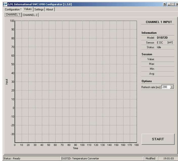
The fields “Model” and “Sensor” are filled in by the software that recognizes the unit that is connected at that moment. By pressing the “START” Button, the SWC1090 will interrogate the unit for its current Input value at a user-selectable refresh rate (Options).
