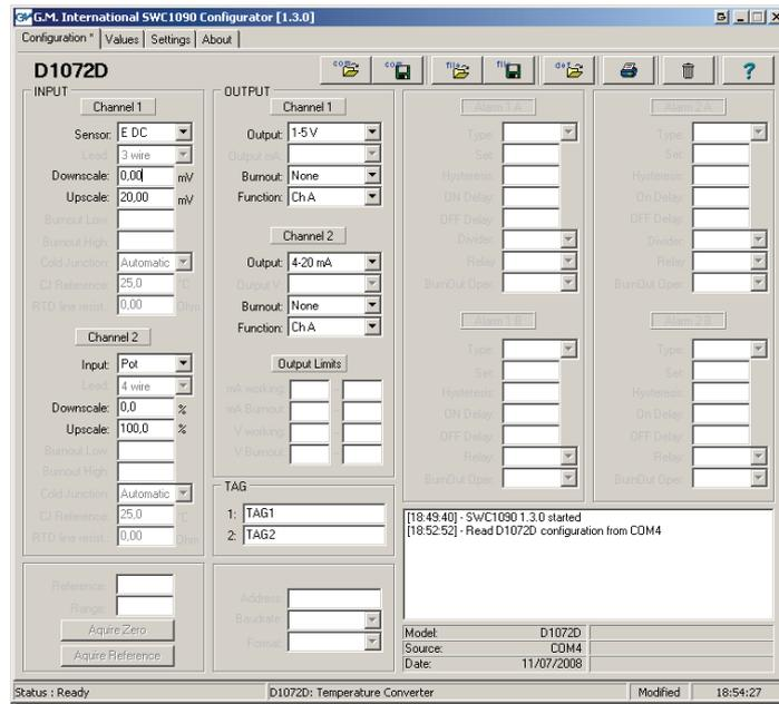
The “Configuration” Tab is the main interface that allows to create and modify configurations. Parameters can be loaded to screen in three ways:
